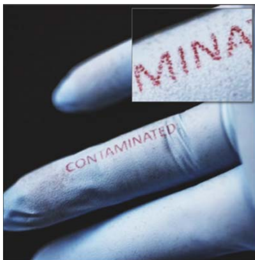
FIGURE 2 Surgical gloves with printed patterns turning to red, showing 'CONTAMINATED', after exposure to Escherichia coli at a concentration of \approx 10^4 CFU/mL, indicating contamination. From H. Tao, B. Marelli, M. Yang, B. An, M.S. Onses, J.A. Rogers, et al. Adv. Mater. 27 (2015) 4273–4279. Copyright Wiley-VCH Verlag GmbH & Co. KGaA. Reproduced with permission.
