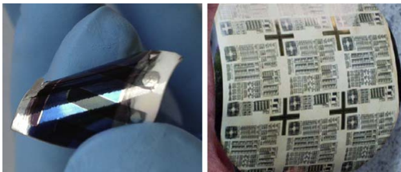
FIGURE 3 (Left) 4% efficient organic solar cells fabricated on paper substrates with a zinc coating acting as the back contact and evaporated MoO 3 /Ag/MoO 3 semitransparent top electrodes. (From L. Leonat, M.S. White, E.D. Głowacki, M.C. Scharber, T. Zillger, J. Rühling, et al. J. Phys. Chem. C . 118 (2014) 16813–16817. Copyright American Chemical Society Reproduced with permission.) (Right) Organic field-effect transistors (OFETs) and integrated circuits on paper substrates. (From F. Eder, H. Klauk, M. Halik, U. Zschieschang, G. Schmid, C. Dehm, Appl. Phys. Lett. 84 (2004) 2673. Copyright American Institute of Physics. Reproduced with permission. Colour image courtesy of Hagen Klauk.)
