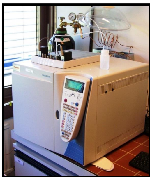
Figure 25. Photo of the Thermo Scientific Trace GC Ultra (on the left) and two typical chromatograms (overlaid) showing the detectable products.
