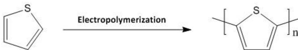
Scheme 4. Schematic representation of the electropolymerization of thiophene to poly(thiophene).
