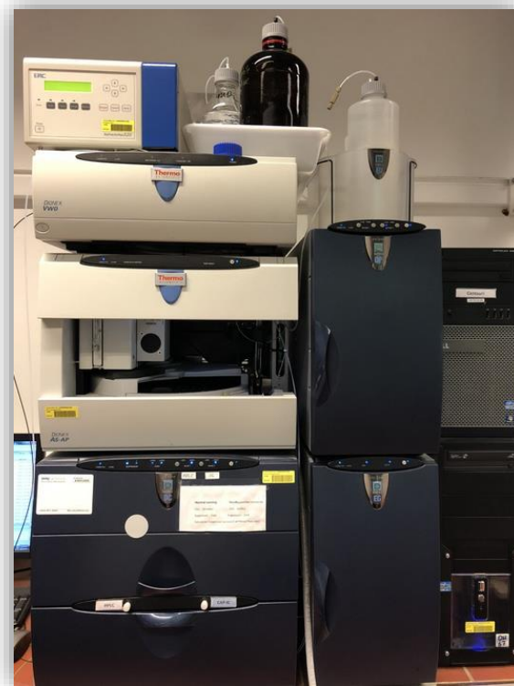
Figure 16. A photo of the Capillary Ion Chromatography for the detection of anionic compounds.
