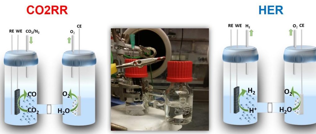
Figure 13. Electrochemical setup for CO 2 RR (left) and HER (right) experiments in an H-Cell configuration. Reprinted/modified from 59 . ©
