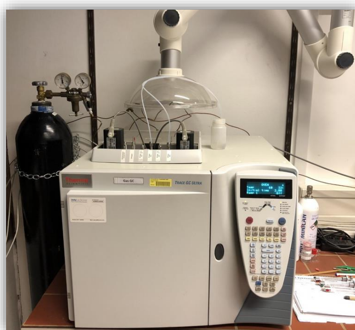
Figure 15. A photo of the Gas Chromatography employed for the analysis of gaseous products (i.e CO and H 2 ).
