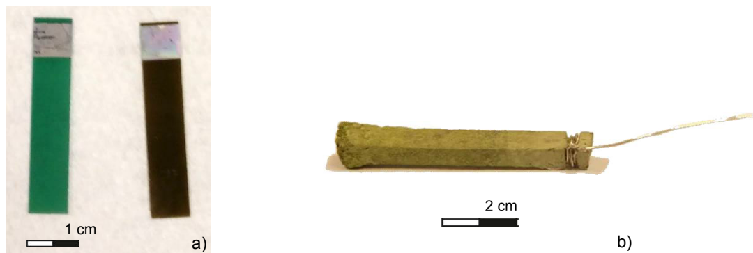
Figure 9: a) 6H-SiC (left) and 4H-SiC (right) with annealed Nickel contacts, b) contacted 3C-SiC sample.
