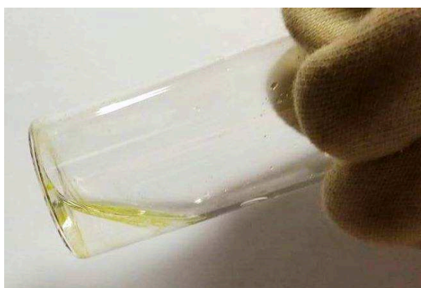
Figure 29: The hydrophobic catalyst Re(bipy)(CO) 3 Cl is not soluble in water, therefore homogenous approaches are only possible in organic electrolytes.
