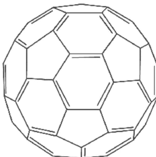
Figure 10: Chemical structure of Buckminsterfullerene ( C_{60} ).
