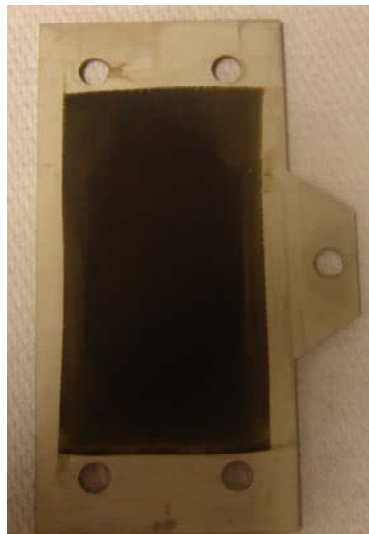
Figure 4.32 Catalyst coated Pt/Ti electrode after 1 h of anode operation in a 3 chamber electrolysis.
