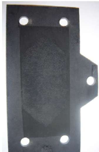
Figure 4.35 Catalytic film coated DSA electrode operated as anode with 5 mA/cm 2 for 1 h.
