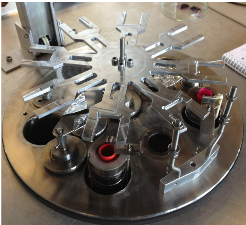
Figure 10. Two-source HWE system with rotating sample carousel. The source shutters are both open.
