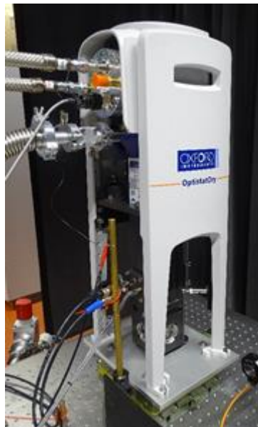
Figure 7: Oxford Instrument cryostat with helium in- and outlet (top) and vacuum connection (bottom).
