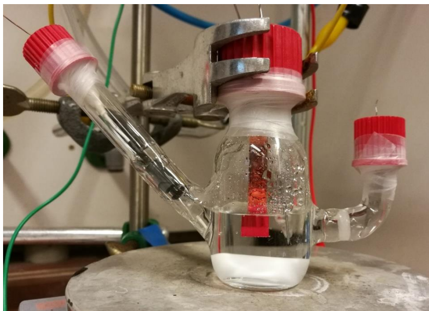
Figure 7: Utilized electrochemical cell for CV measurements in aqueous electrolyte with a Ag/AgCl/3M KCl reference electrode (RE) (left), Pt-foil as counter electrode (CE) (right), and a PTCDa/Cr-Au working electrode (WE) (middle).
