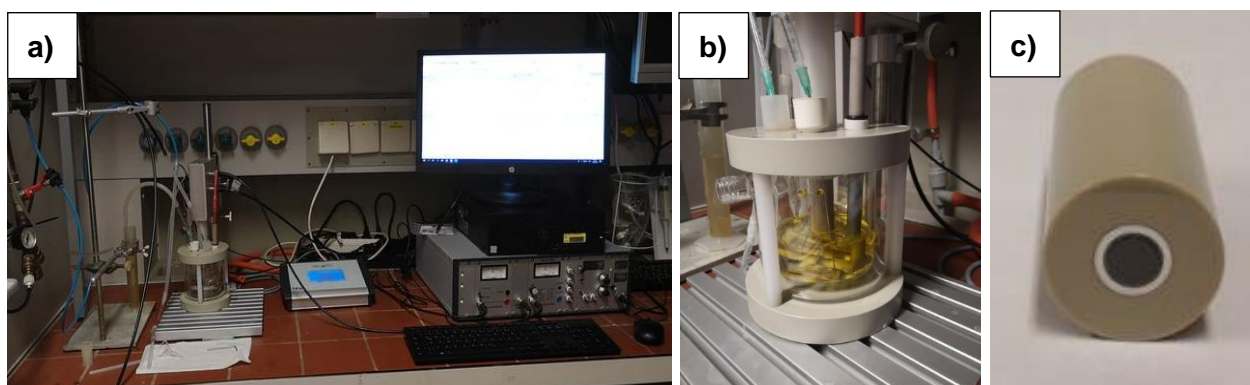
Figure 10: a) Setup for RDE and RRDE measurements with the bipotentiostat, rotator as well as rotation controller. b) Purging an electrolyte solution in the glass compartment with the electrode attached to the rotator. c) Picture of the GC/Pt RRDE.
