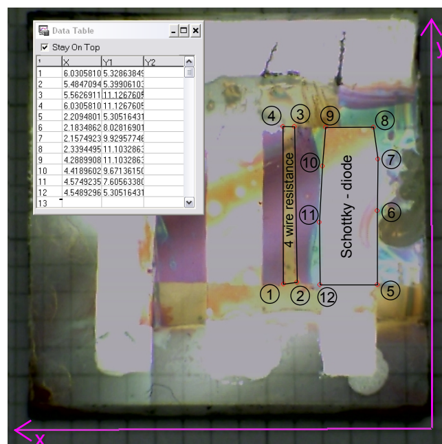
Figure 2.7: Picture of solar cell device. The picture was taken with reflecting light, to make the ITO layer visible. The active area of the Schottky-diode and the 4 wire resistor are shown with their coordinates in x and y axis.
