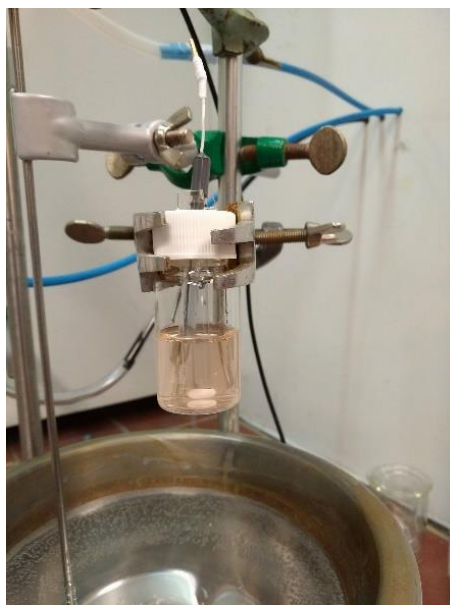
Figure 5: Set up for electrodeposition of ZnO/eosin Y.
