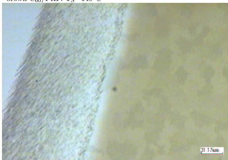
FIGURE 4.6. Sample mcp07: Light microscope picture of C_{60} /PHP bilayer on mica in trough-light geometry. Left PHP, brown C_{60} /PHP. T_S=90^\circ\text{C}
