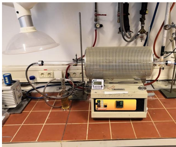
Figure 4: Tube furnace connected with N 2 supply and gas washing bottle
