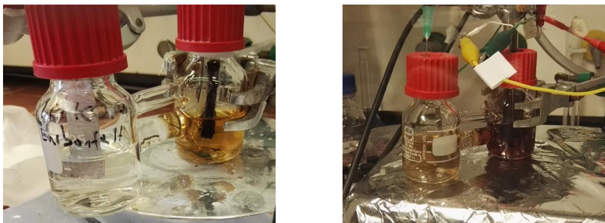
Figure 29: (left) cell with PDA on CF as working electrode after 48 h chronoamperometry in 1M KOH (right) cell with CF as working electrode after 70 h chronoamperometry in 1M KOH
