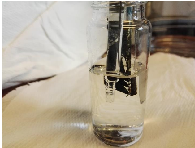
Figure 23: Delamination of PDA film of FTO glass after 100 cycles cyclic voltammetry
