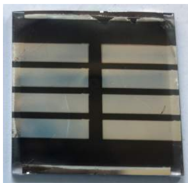
Figure 7: 8 completed perovskite solar cells consisting of (from bottom to top: An ITO-glass, a PTAA hole transport layer, a wide-band gap perovskite layer, a C_{60} electron transport layer, a BCP buffer layer and Ag electrode contacts).
