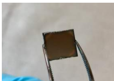
Figure 8: Double-cation perovskite film on quartz glass with the composition \text{FA}_{0.8}\text{Cs}_{0.2}\text{Pb}(\text{I}_{0.6}\text{Br}_{0.4})_3 processed by spin coating.
