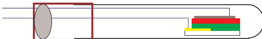
Figure 3.10: Encapsulated sample for a PCDMR measurement
