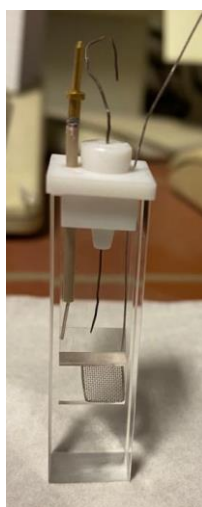
Figure 7: Spectro-electrochemical cell with Pt-mesh as WE, Pt wire as CE, and \text{Ag}/\text{AgCl} as quasi RE.
