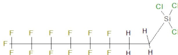
Figure 1.3.8: Structure of tridecafluoro-(1,1,2,2-tetrahydrooctyl)-trichlorosilane
