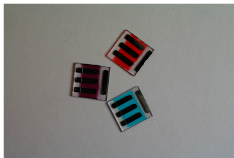
Figure 1.3.1: Devices using different semiconductors. violet: P3HT, red-orange: MDMO-PPV, blue: ZnPc
