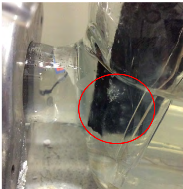
Figure 20 Biofilm formed after proceeding growth of the microorganisms on the electrode for 3 days. The red circle displays the microorganisms grown on the electrode.
