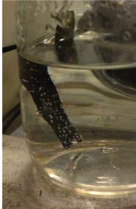
Figure 40 Oxygen evolution on the surface of the Nocera catalyst electrode due to catalyzed oxidative water splitting reaction in the anode compartment of MEC1.
