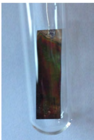
Figure 36 Photograph of the obtained Pt electrode covered with Nocera catalyst after electropolymerization procedure.
