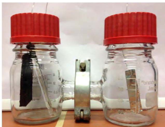
Figure 10 Microbial electrolysis cell. Photograph on the left hand side and schematic of the cell on the right hand side display the setup used. Setup shows anode compartment (right) and cathode compartment (left) separated by membrane which was fixed between the compartments using a clamp. Electrical contacts for the electrodes as well as gas in- and outlets were implemented via septa.
