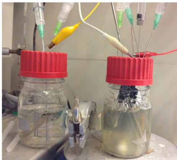
Figure 11 Microbial electrolysis cell after inoculation of sewage suspension containing microorganism to the cathode compartment (right-hand side).
