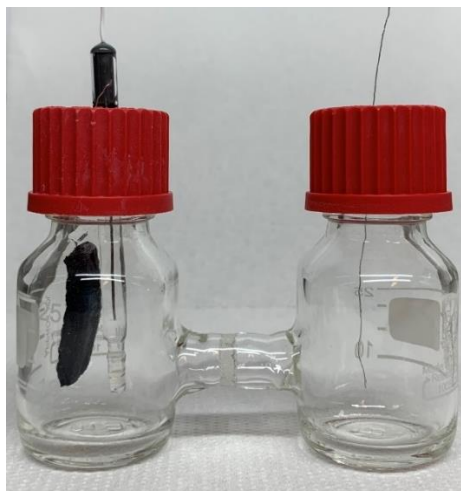
Figure 28. A photo of a setup for enzymatic electrolysis experiments.
