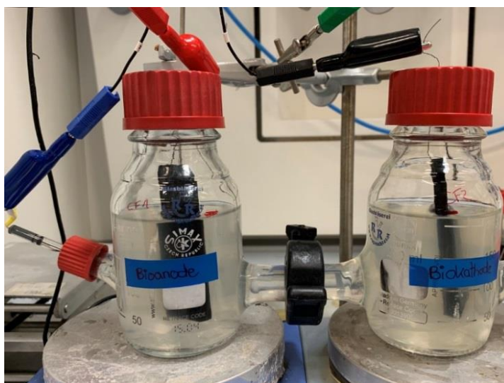
Figure 21. A photograph of two-compartment microbial electrolysis cell containing a bioanode and a biocathode.
