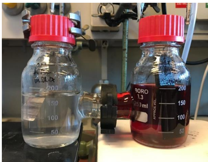
Figure 42. A photo of MEC 2 containing 50 \mu\text{M} neutral red in cathodic electrolyte solution
