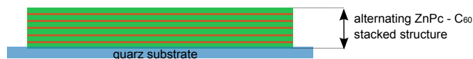
Figure 2.15: Heterojunctions applied to the photoinduced absorption setup in the mid-infrared region. For the reflexion element in ATR mode a germanium crystal is used. ZnPc is photoexcited from the top side.
