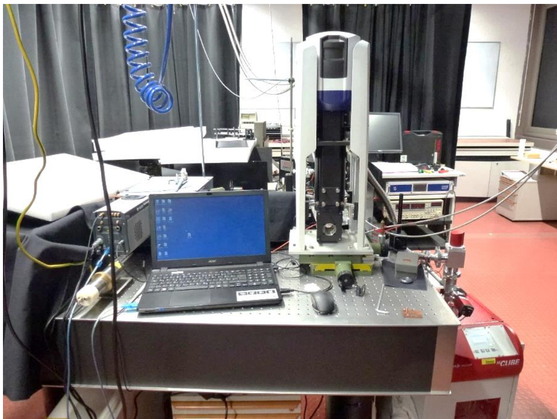
Figure 2.4: Photoluminescence (PL) and photoluminescence decay (PLD) set-up.
