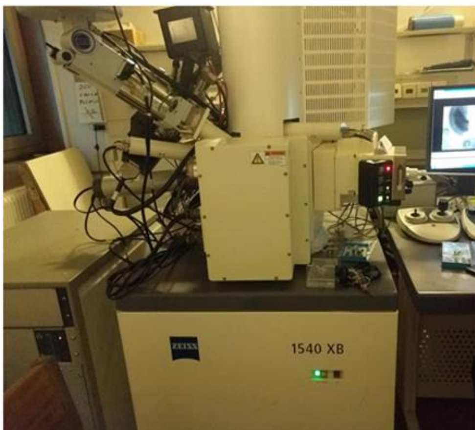
Figure 2.7: Image of a scanning electron microscope (SEM, ZEISS 1540 XB cross-beam scanning microscope equipped with a focused ion-beam (FIB) unit).
