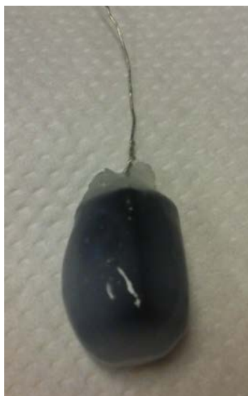
Figure 13: Carbonfelt Electrode covered with Enzyme - Alginate layer.
