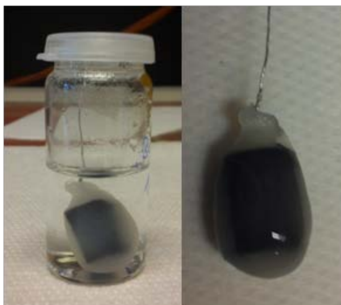
Figure 25: CF/Alginate/ F_{ate}DH / F_{ald}DH /ADH electrode after 4 weeks storage in 18 M \Omega water.
