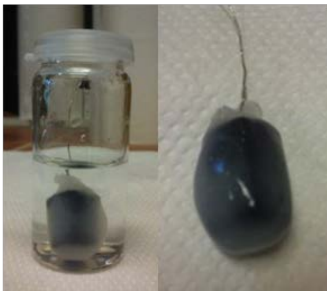
Figure 24: CF/Alginate/ F_{ate}DH / F_{ald}DH /ADH electrode after 3 weeks storage in 18 M \Omega water.
