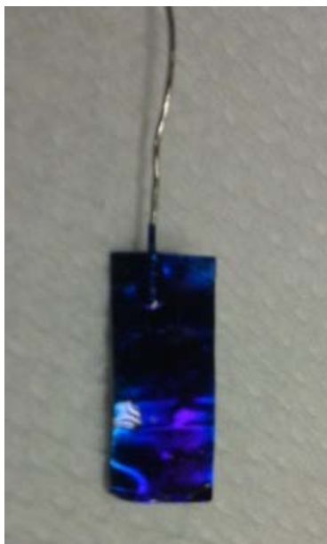
Figure 15: Platinum electrode covered with a thin layer of polypyrrole with incorporated enzyme.
