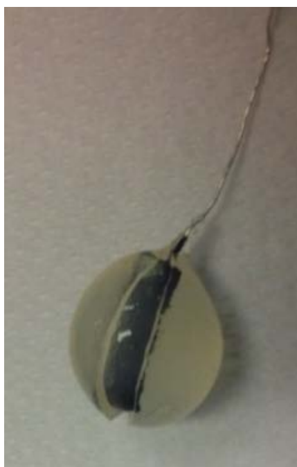
Figure 32: Pt electrode modified with polypyrrole film and an alginate layer containing F ate DH with crack in the alginate layer formed during electrolysis.
