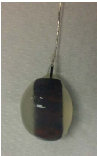
Figure 14: Platinum Electrode covered with a film of polypyrrole and an Alginate - Enzyme layer.
