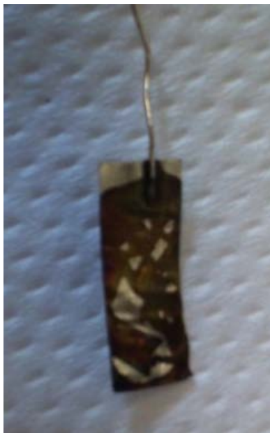
Figure 40: Pt/PPy/ F_{ate}DH electrode after electrolysis. At some places the PPy film was peeled away.
