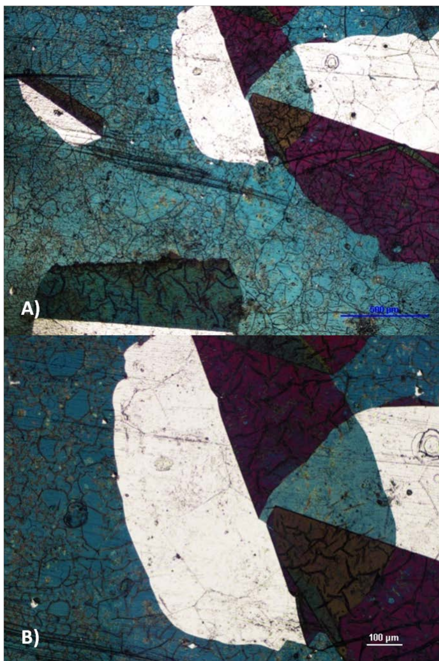
Figure 43: Pt/PPy electrode without enzyme modification after electrolysis at 500x magnification (A) and 1000x magnification (B). The polypyrrole film was peeled off during electrolysis at some points of the electrode.
