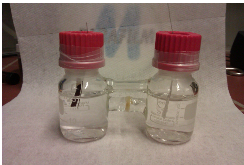
Figure 14: H-cell for electrolysis. The cell contains a WE (Pt-plate with polymeric film) and a Ag/AgCl-quasi RE on the one side of the cell and on the other side a CE (Pt-plate).
