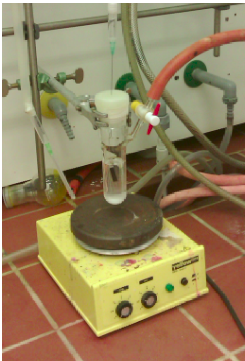
Figure 24: Complexation of poly-4-methyl-4'-(3-thienylheptyl)-2,2'-bipyridine film with \text{Re}(\text{CO})_5\text{Cl} in hot toluene.
