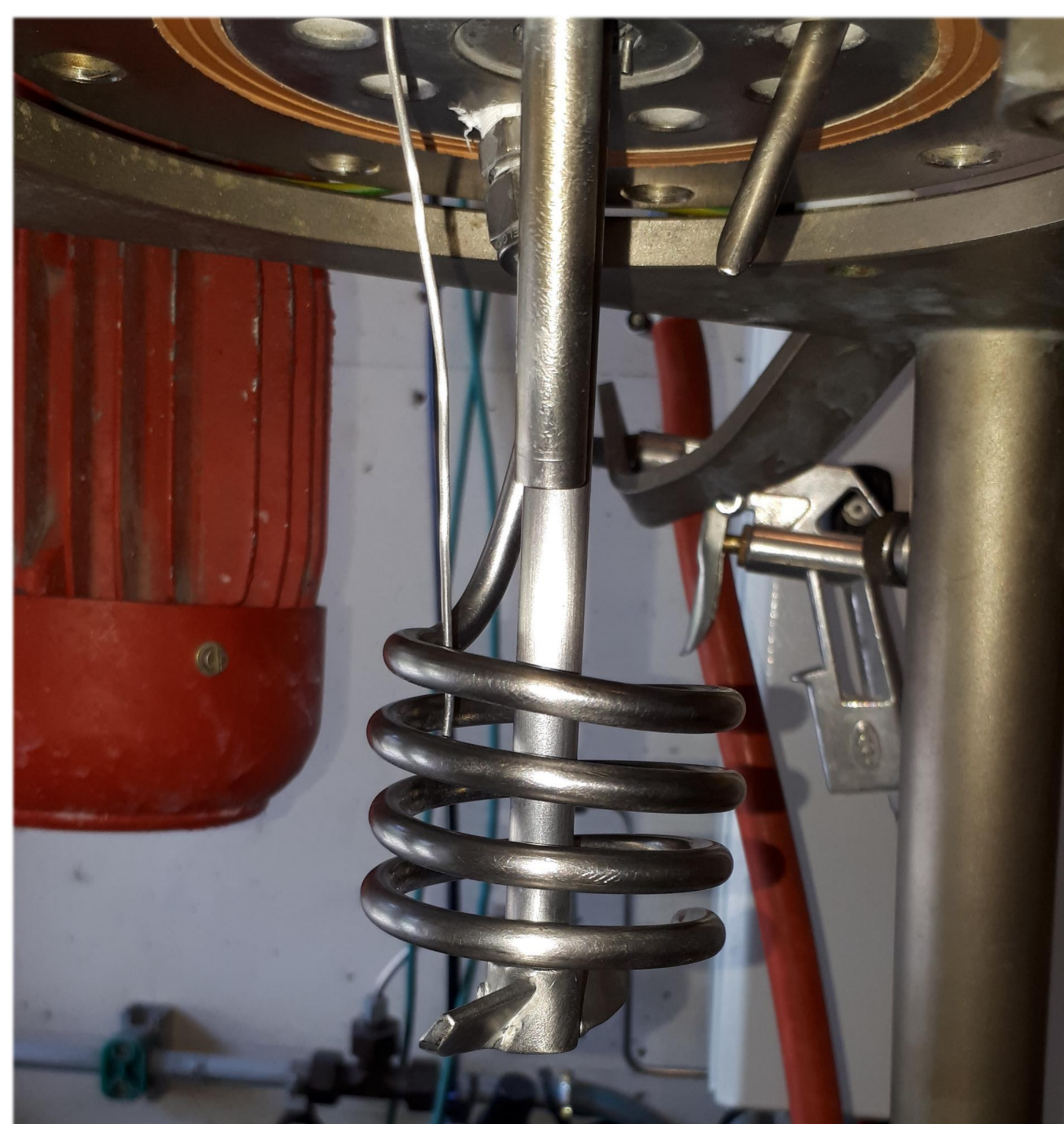
Figure 2: The internal heating coil compensates for heat loss or heat build-up.
