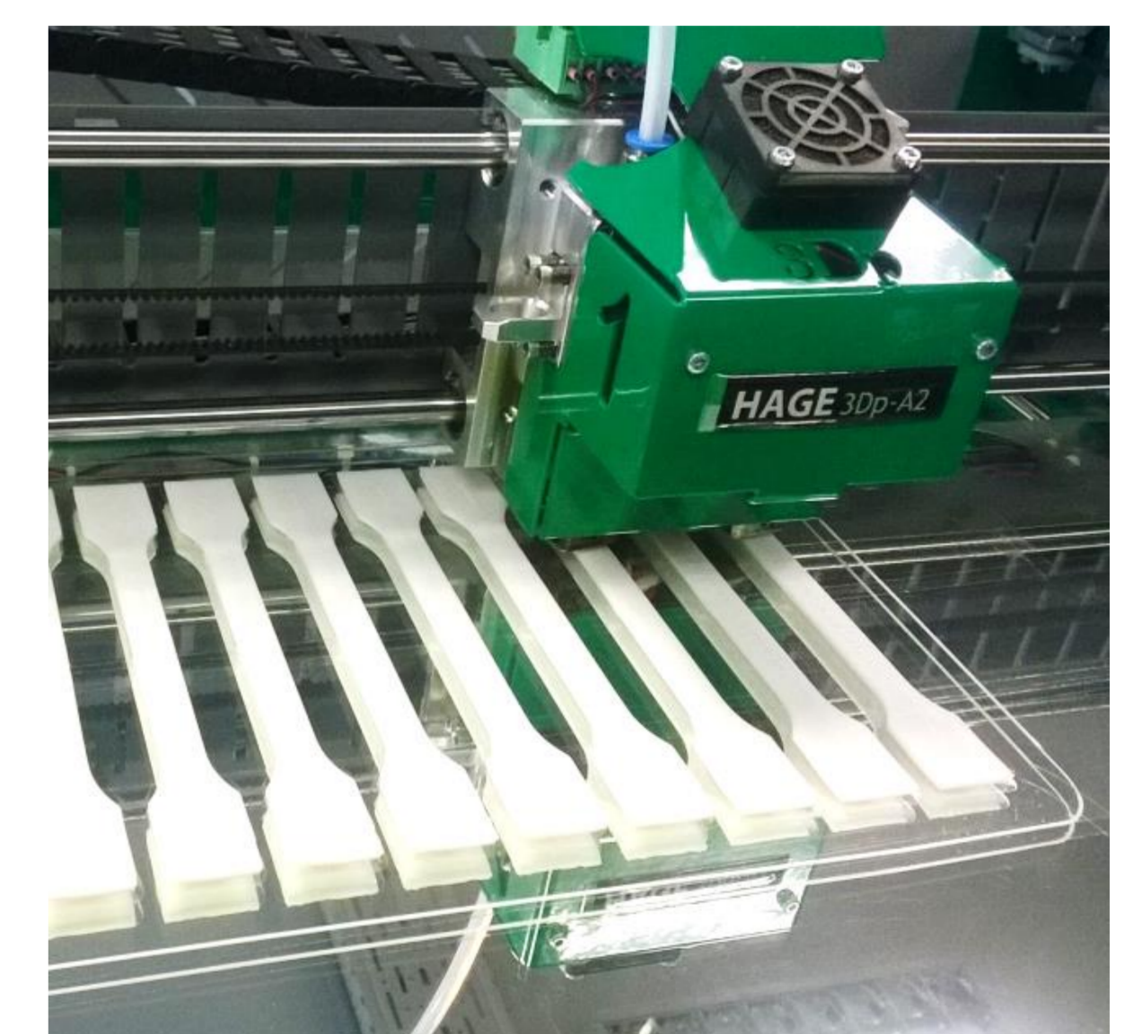
Figure 4: Surface plot of Viscosity \eta_0 (left) and FFF-printing of tensile test shoulderbars (right).
