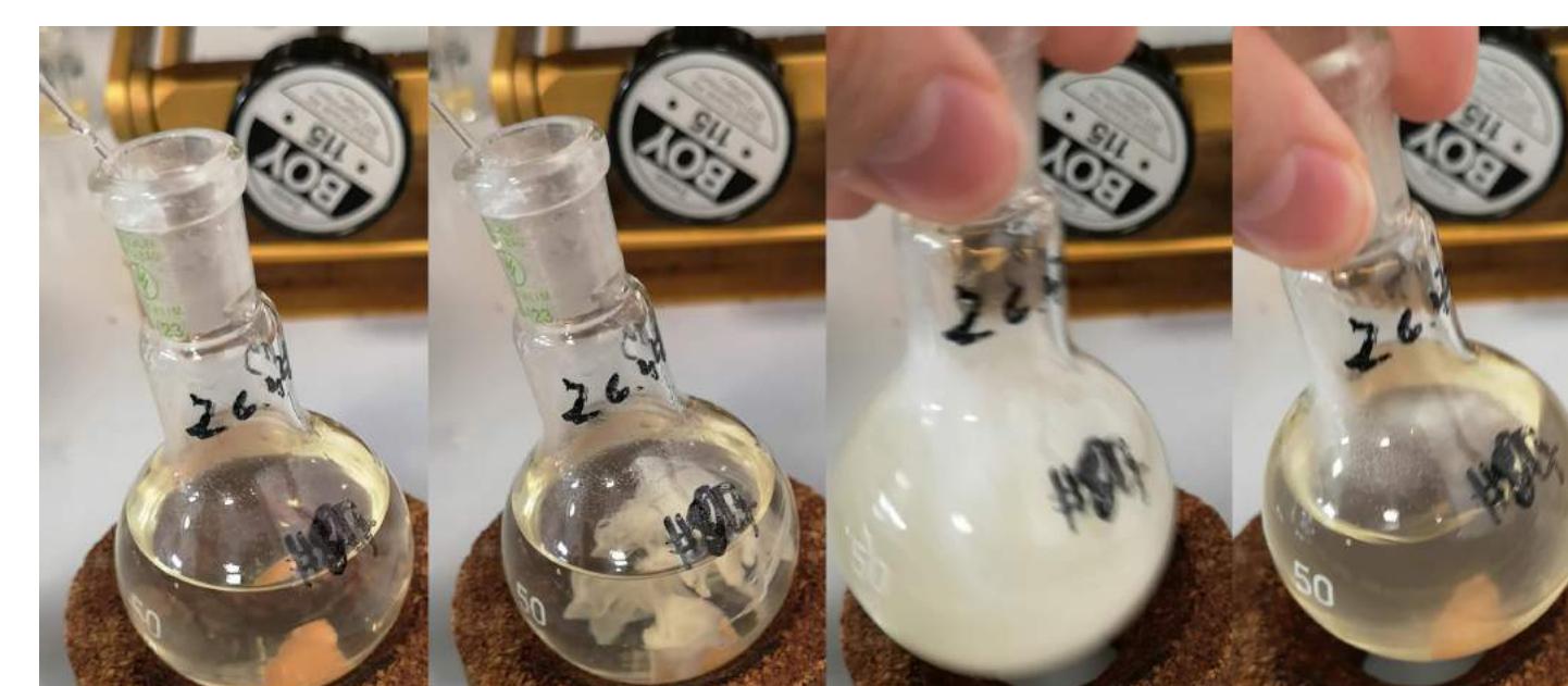
Fig. 3 - The change of polymer solubility with the addition of a drop of hydrochloric acid to an alkaline polymer solution.
