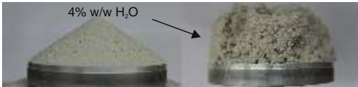
Fig.1: Creation of cavities in sand sample by adding water. Left dry sample and right wet sample.
