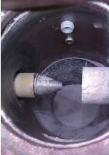
Fig.2: Nozzle and conveying duct of the feeding injector
