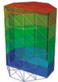
Fig.2: (a) Grid used for averaging and coupling of granular properties. (b) Surface of the grid used to measure the mass flow into and out of the fg Sub-region.
