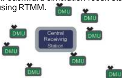
Fig.3: Concept of a swarm of small autonomous dust measurement units for local emission or immission measurements
