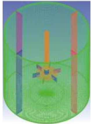
Fig.1: Stirred tank reactor mesh
