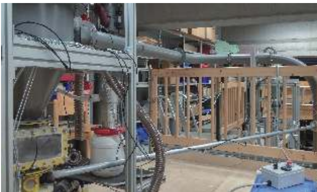
Fig.2: Cyclone with attached particle feeding injector to operate a closed loop dust recycling system
