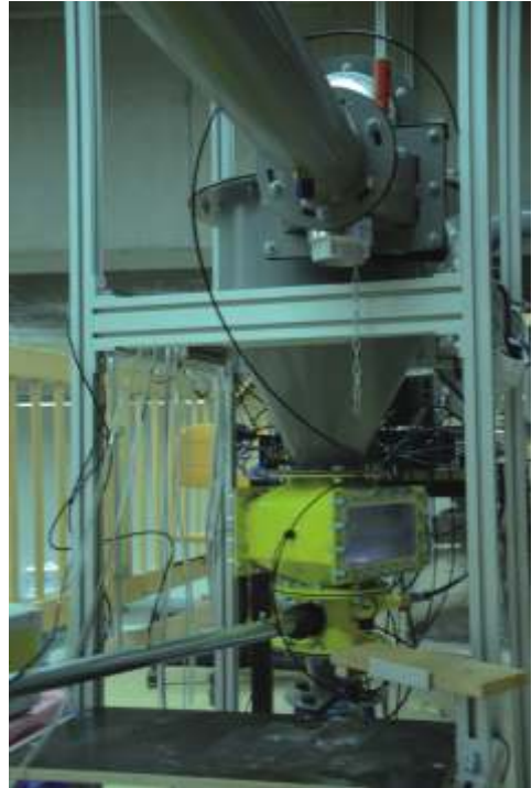
Fig.3: Nozzle and conveying duct of the feeding injector
