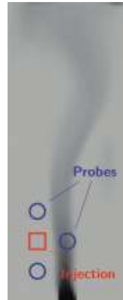
Fig.1: Recurrence plot (left) of a CFD simulation of an oscillating bubble column (right); in the right figure tracer probes are depicted
