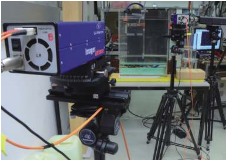
Fig.1: Two camera PIV setup to acquire flow field data at different spatial resolutions simultaneously.
