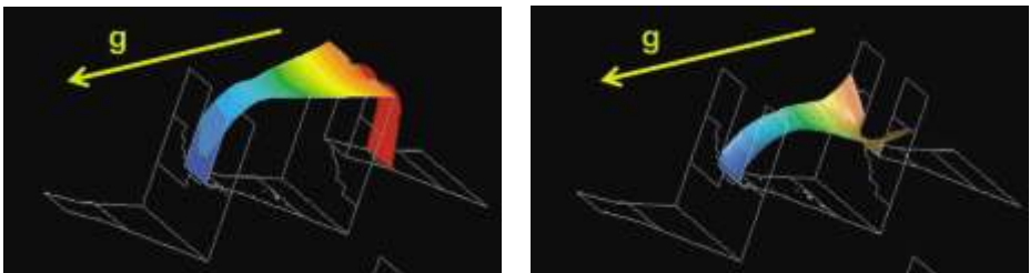
Fig.2: Numerical simulation of liquid transport in complex microchannels. The images display the moment the interface reaches the sharp edges from both sides (left), and the moment the interface is pinned at one edge and moves on the other edge (right). This flow behaviour has application in uni-directional liquid transport through microfluidic devices.
