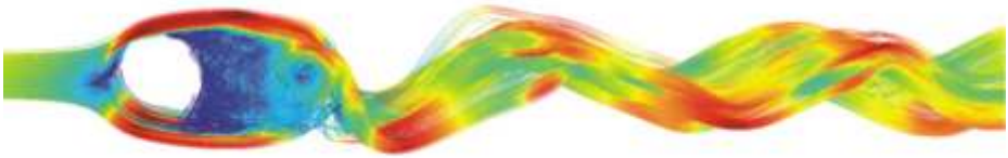
Fig.1: Streamlines of the turbulent flow past cylinder at Re=3900 . The red color refers to the highest velocity, and the dark blue colors the lowest.
