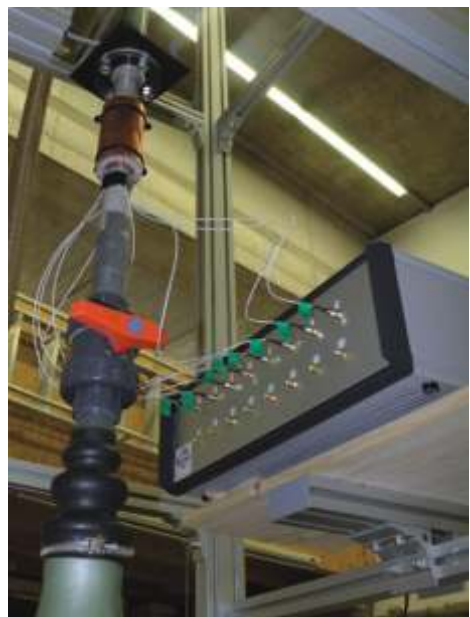
Fig.2: Single plane ECT sensor on our hopper discharge experiment in the PFM lab. The grey box is the main hardware unit of the ECT system which sends its raw data via network connection to a PC running Matlab for three-dimensional data reconstruction.
