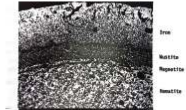
Fig.2a : Snapshot of a sintered iron ore pellet reduced 30%, where every layer with various pore structures are visible [4].
