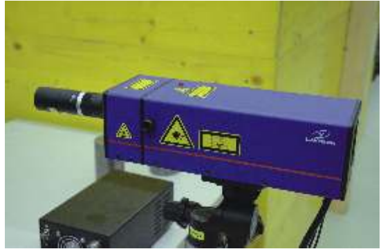
Fig.1: New CW Laser for time resolved PIV and a snapshot of shear layer turbulence in a free jet.
