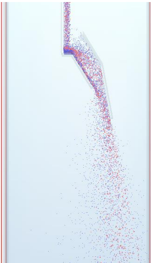
Example of a experimental simulation validation: Lab-scale charging experiment (left) and corresponding DEM simulation (right)
