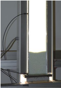
Fig. 1: Fluidized bed test rig with background illumination
