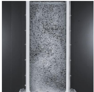
Fig. 2: Still image of high-speed video. The bubble column is aerated through a porous plate at the bottom.
