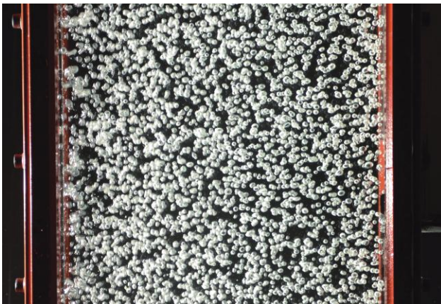
Fig. 3: Detail view of the inlet section of the bubble column. Bubbles of similar size are rather uniformly distributed in lateral direction.
