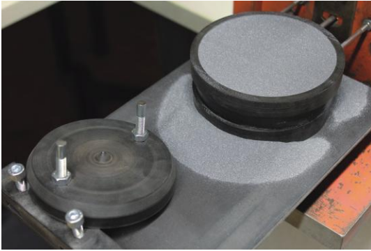
Fig. 3: Shear cell depicted in the left. In the right top result of calibration without cohesion for artificially high friction parameters. Right bottom result of calibration process incorporating cohesion and using intermediate realistic friction parameters.
