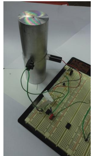
Fig. 3: Prototype of the optical detection unit.
