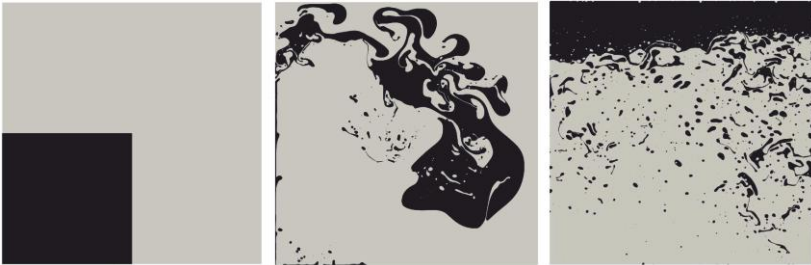
Fig.1: Highly-resolved numerical simulation of interfacial turbulence in the phase inversion problem. The images display liquid-liquid interfaces at different stages of the problem.
