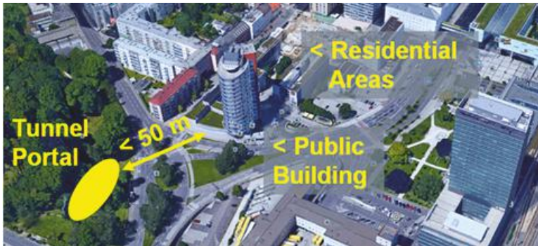
Fig.1: Linz/Westring configuration, showing a point-source of pollutants (future tunnel portal, marked by yellow ellipse), a bluff body obstacle (public building Wissensturm) and a residential area (in the wake of Wissensturm).
