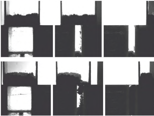
Fig.2: To test our hypothesis of a local fracture formation, we have artificially applied discrete vertical forces strings to the initial powder bulk. We can observe a substantial increase of the disposed material (right).
