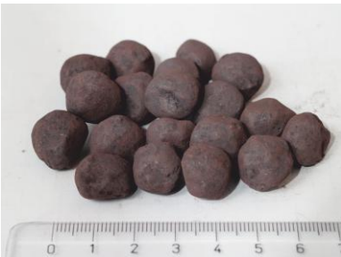
Fig.2: Pelletized iron ore with scale (by Arnoldius (CC BY-SA))
