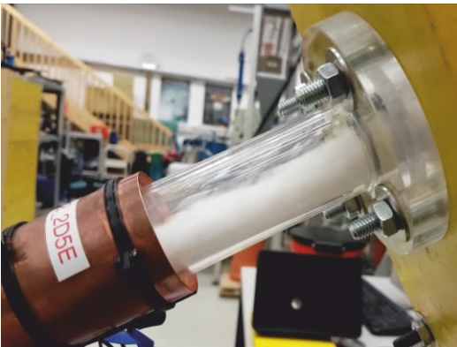
Fig.1: Snapshot of the new lab test rig to investigate particle flows in pipes. The setup can be tilted from a vertical to a complete horizontal position and by pressurizing the storage hopper we can modulate the height of the particle strand.
