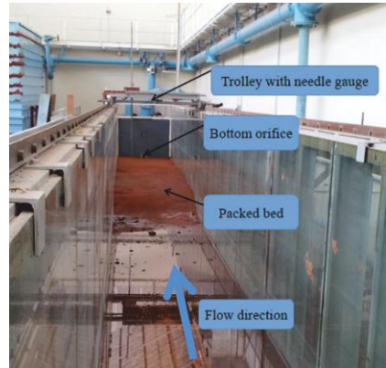
Fig.2: Experimental setup of bottom outlet flushing process in reservoirs [1].
