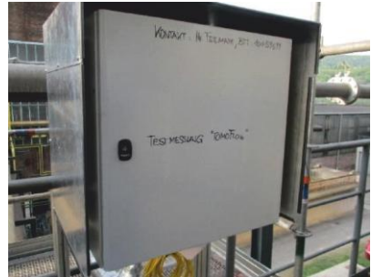
Fig.1: Sensor and signal processing unit installed at the main pipe for pulverized coal transport at voestalpine Linz. The pipe diameter is 150mm and operating temperatures are around 80°C (due to the pre-conditioning of the coal), thus temperature stability of the sensor and electronics is an important issue.
