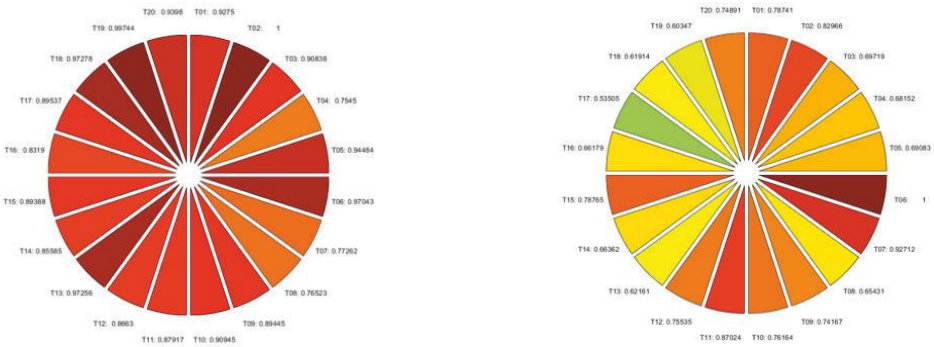
Fig. 2: Long term statistics of BF1 (left) and BF 4 (right) at voestalpine Donawitz for approx. 6500 hours of blast furnace operation. The numbers of detected blockages is given on a relative scale. While BF1 shows a more even distribution of blockages along the different tuyeres, BF4 has some tuyeres with a higher blockage frequency.
