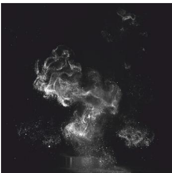
Fig.2: Reconstruction of particle distribution inside the pipe, recorded at 100Hz. The data clearly shows an unsteady transport mode (slug flow).
