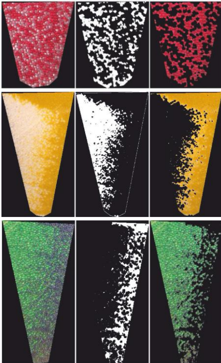
Fig.2: Examples of image processing results to separate particle classes of different size and colour.
