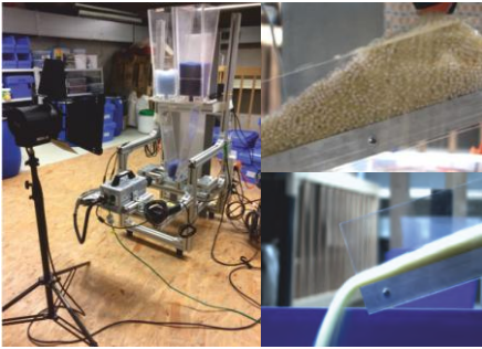
Fig.1: Images of the experimental setup. On the left we have the mixing of two different particle classes in one hopper. The right images show the mixed hopper discharge onto a chute and the segregation of particles during transport along the chute.
