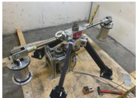
Fig.2: Centrifuge for flowability experiments under increased gravity conditions up to 100G. Test rig assembly at the technology center of RHI-Magnesita in Leoben.
