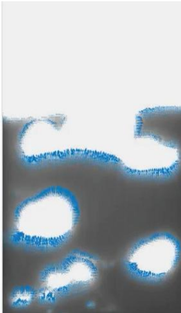
Fig.1: Shadowgraphy recording of a bubbling fluidized bed. The Lucas-Kanade method was used to extract the motion in the video. In this case the optical flow approach serves a kind of front-tracking method. A quick quantitative comparison of the bubble rise velocities with formerly calculated results based on Lagrangian object tracking of the bubbles shows a good agreement in bubble rise velocities (c.f. figure below, the vector data is completely unfiltered and still shows a realistic range of bubble rise velocities).
