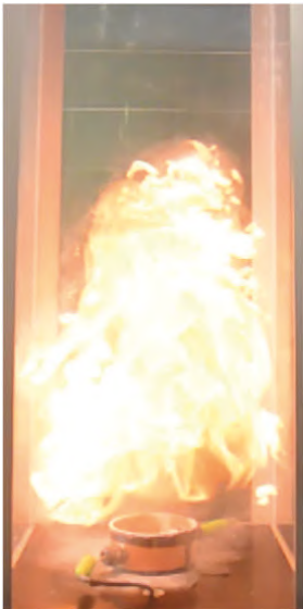
Fig.1: Image series of a dust deflagration experiment. To extract the geometry of the flame it is sliced into a sequence of equally spaced layers and for each of these layers the center location and extension of the flame is calculated.
