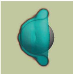
Fig.2: A snapshot of fully resolved VOF-IB simulation of droplet-particle collision at We = 69 .
