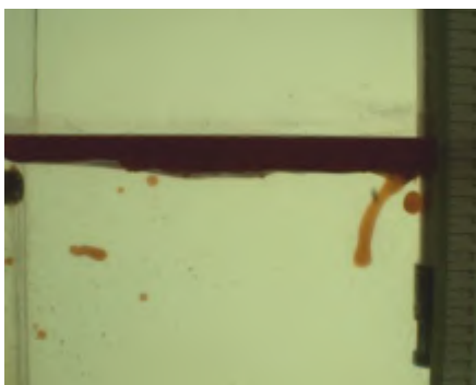
Fig.3: Vortex triggered droplet entrainment around a submerged entry nozzle in asymmetric flow conditions.
