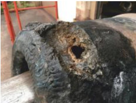
Fig.2: Example of a damaged tuyere. (photo courtesy of voestalpine Donawitz).
