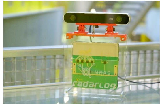
Figure 1 Combination of a radar sensor (bottom) and a stereo camera (top).
